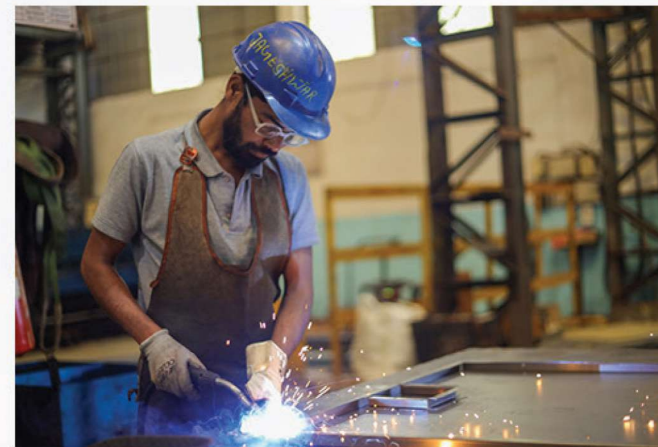
Lift body Manufacturing and MIG Welding Set Up
